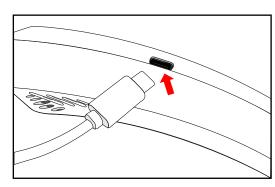
2. Plug large end of USB cable into a USB-Power adapter, laptop, or other device (not included).
