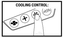
Control high or low cooling output by pressing \*\* button.
